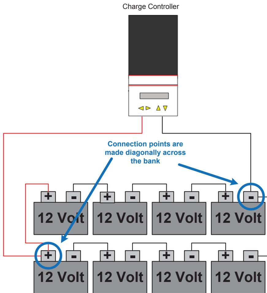
**IMPORTANT:** This is not intended to be a complete system diagram; fusing, disconnects, and grounding should comply with local electric codes.
