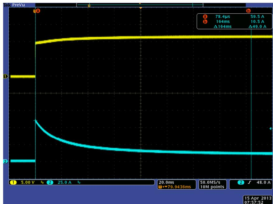
Figure 1. The oscilloscope capture of a SS-10L-12V controller turning on a bank of incandescent lights.
