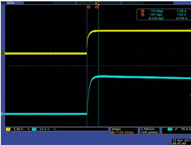
Figure 4. A magnified look at what is happening in Figure 3 when the load turns on (when the yellow goes low-to-high).
