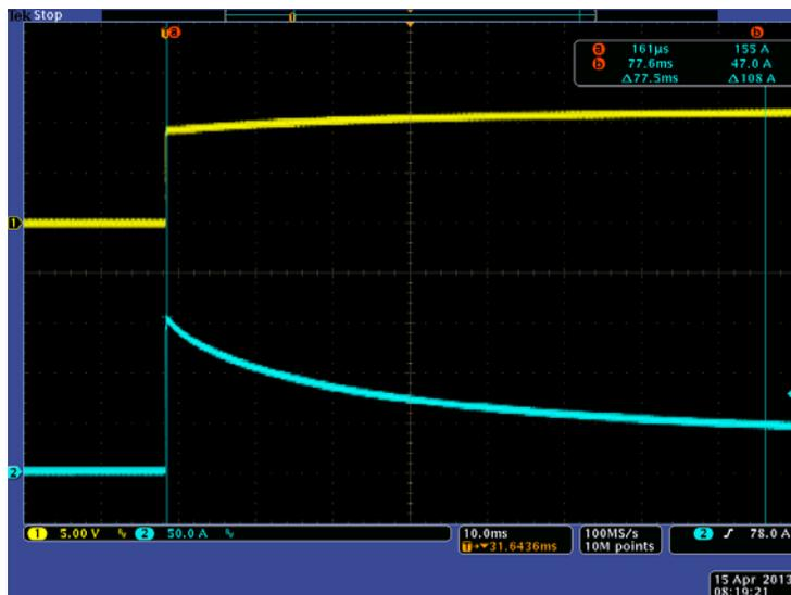
Figure 3. A SS-20L-12V controller turning on a much larger bank of incandescent lights.
