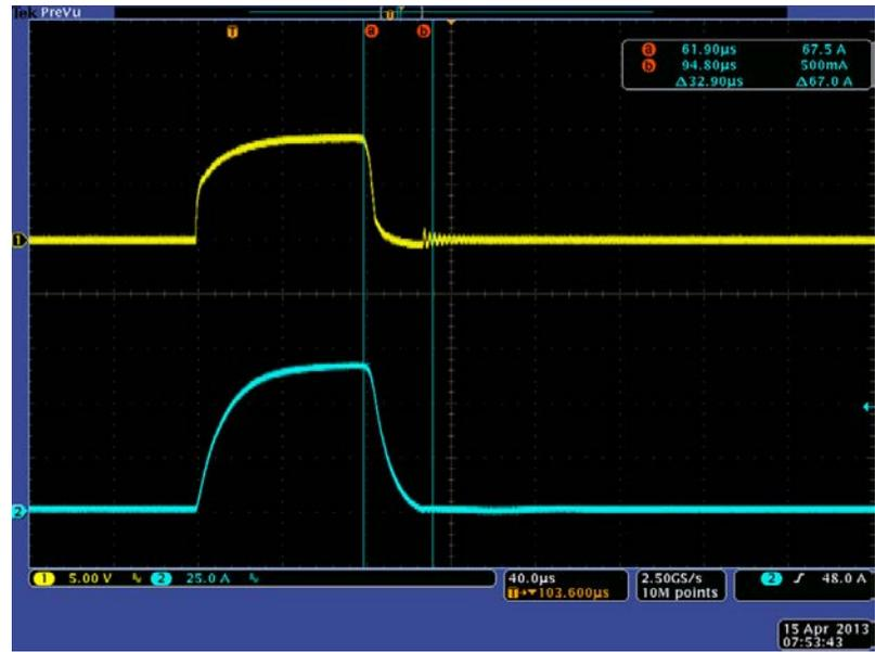
Figure 2. The same SS-10L-12V controller as in Figure 1; this time, a greater number of cold incandescent lights are used than in our Figure 1 test.
