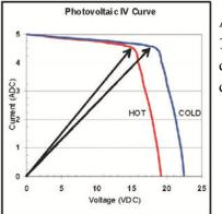
Additionally take note of the module performance IV curves for a 12V nominal PV module. It shows that under the hottest conditions the voltage is still high enough to provide charging current for the batteries.
