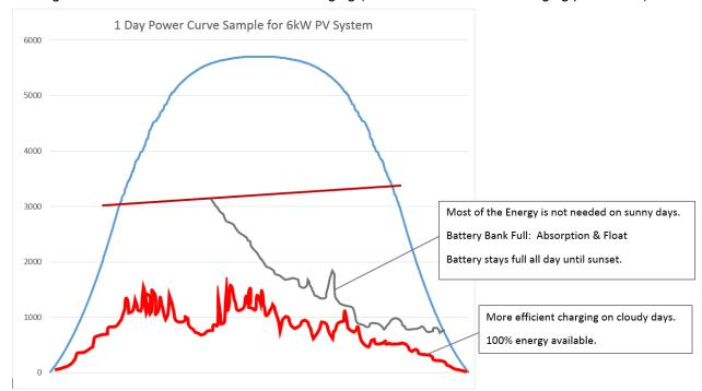
Morningstar's TriStar MPPT 600V Direct DC Charging (red line indicates max. charging power limit)
