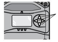
Illuminated arrow buttons indicate which direction(s) are possible on each screen.
