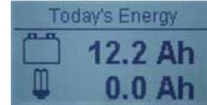
**Battery Icon:** Cumulative Amp-Hours delivered to the battery during today's charge cycle
