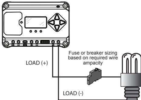
Turn the loads off, and connect the load wires to the load terminals. **DO NOT CLOSE THE FUSE OR BREAKER AT THIS TIME.**
