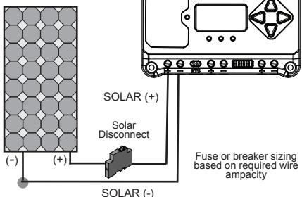
With the solar disconnect open, connect the solar (PV) array wires to the EcoPulse solar terminals. Use caution, since the solar array will produce current whenever in sunlight. **DO NOT CLOSE THE DISCONNECT AT THIS TIME.**
