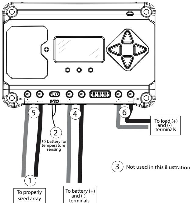
Figure 3-2. Wiring the EcoPulse
