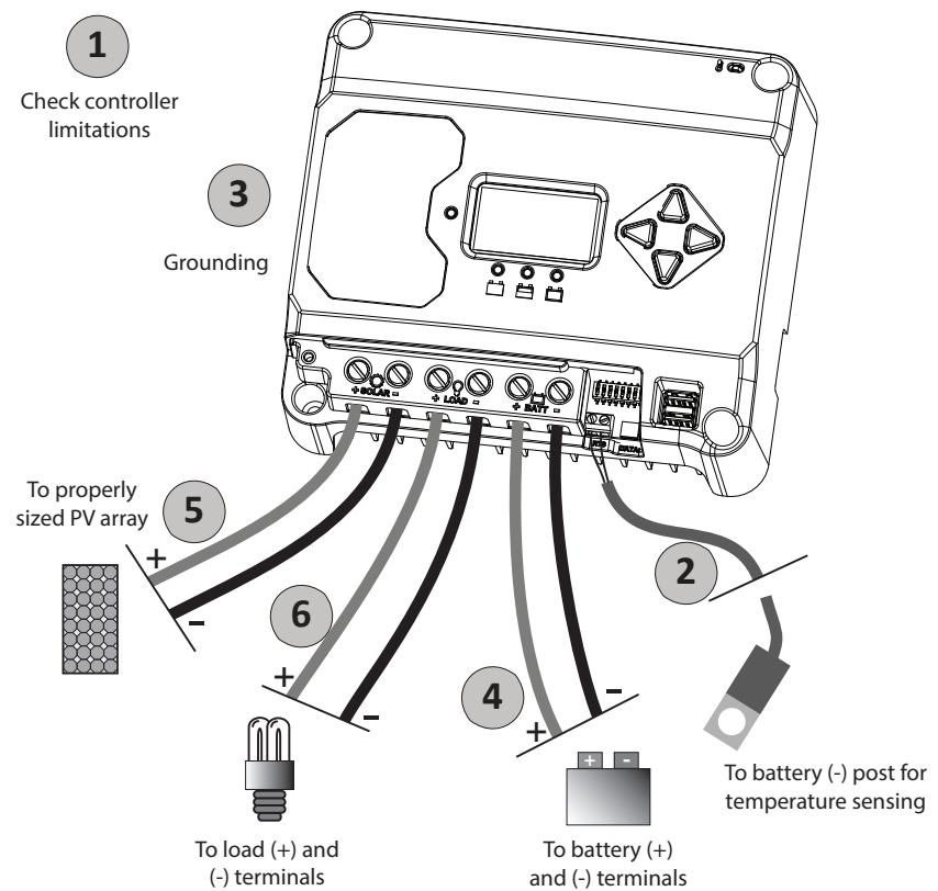
Figure 3-3. Wiring the EcoBoost MPPT
