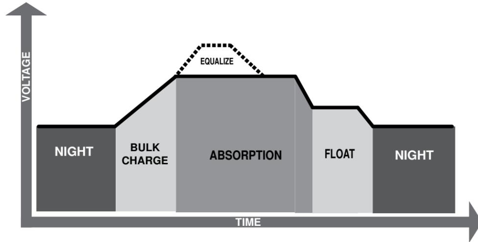
Figure 4-1 TriStar MPPT 600V Charging Algorithm
