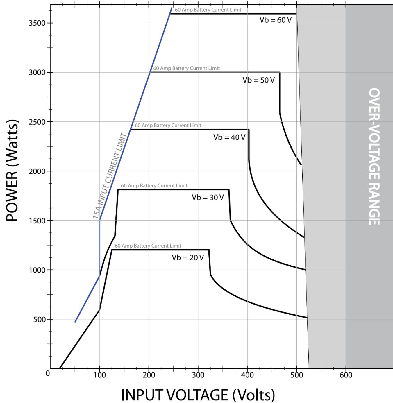
Figure 10-3. Output Power vs. Array Voltage
