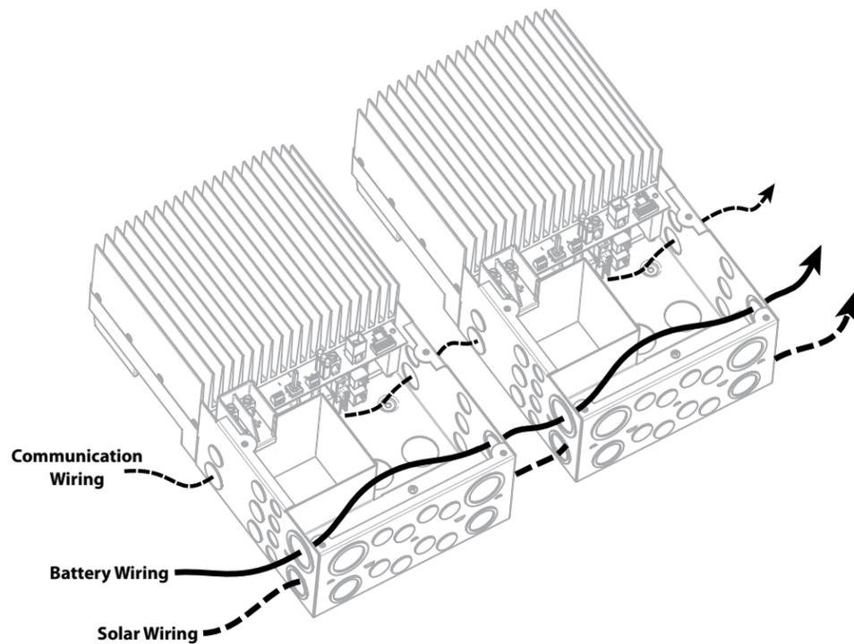
Figure 3-6. Wiring pass-through paths between multiple controllers
