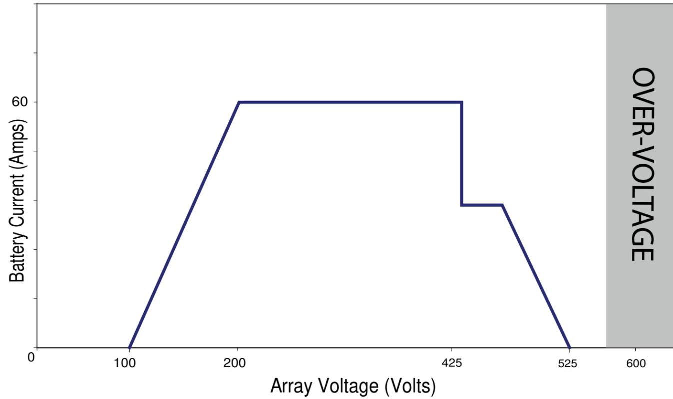
Figure 10-1. Battery Current vs. Array Voltage
