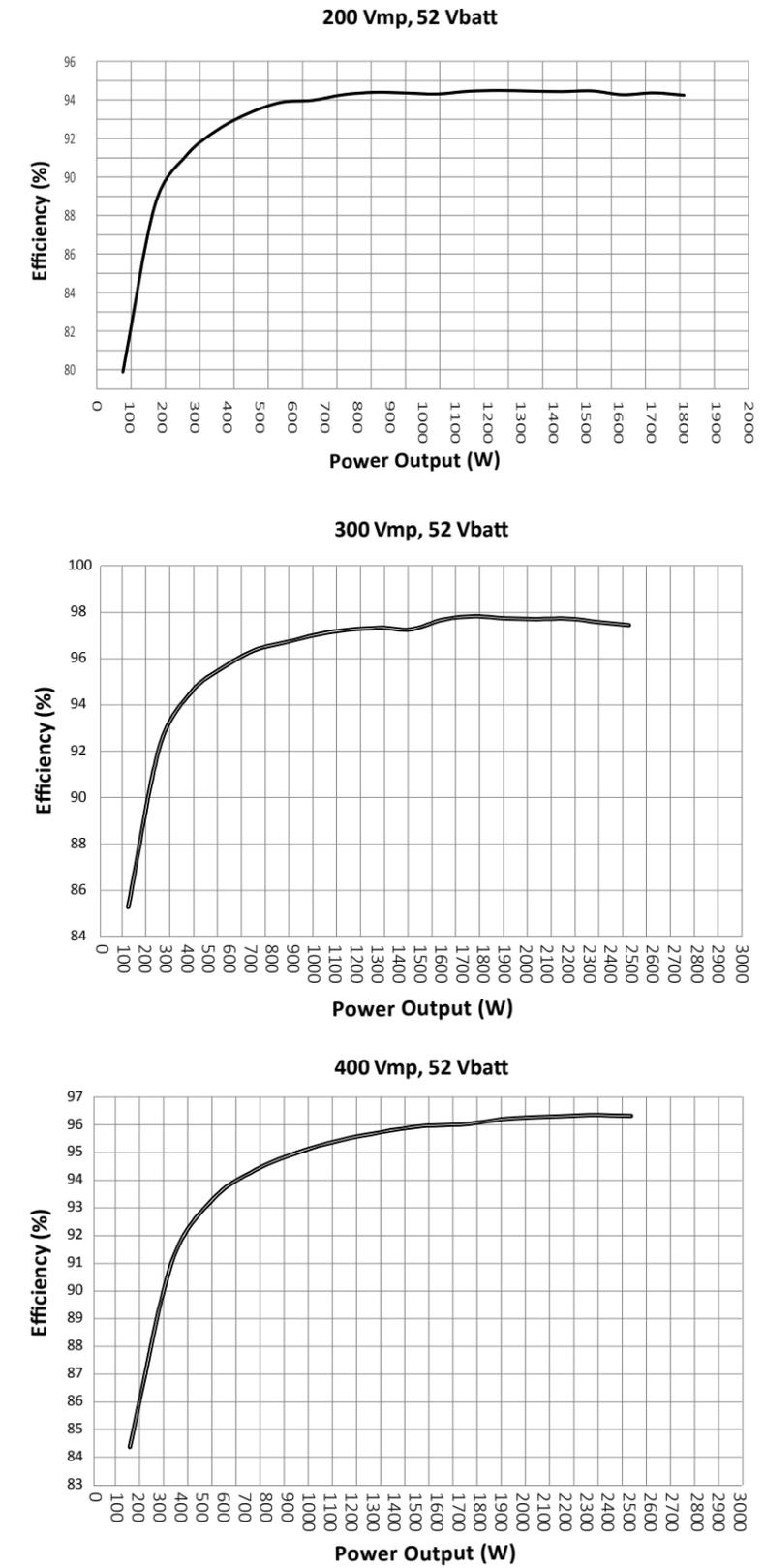
Figure 10-4. Efficiency Curves
