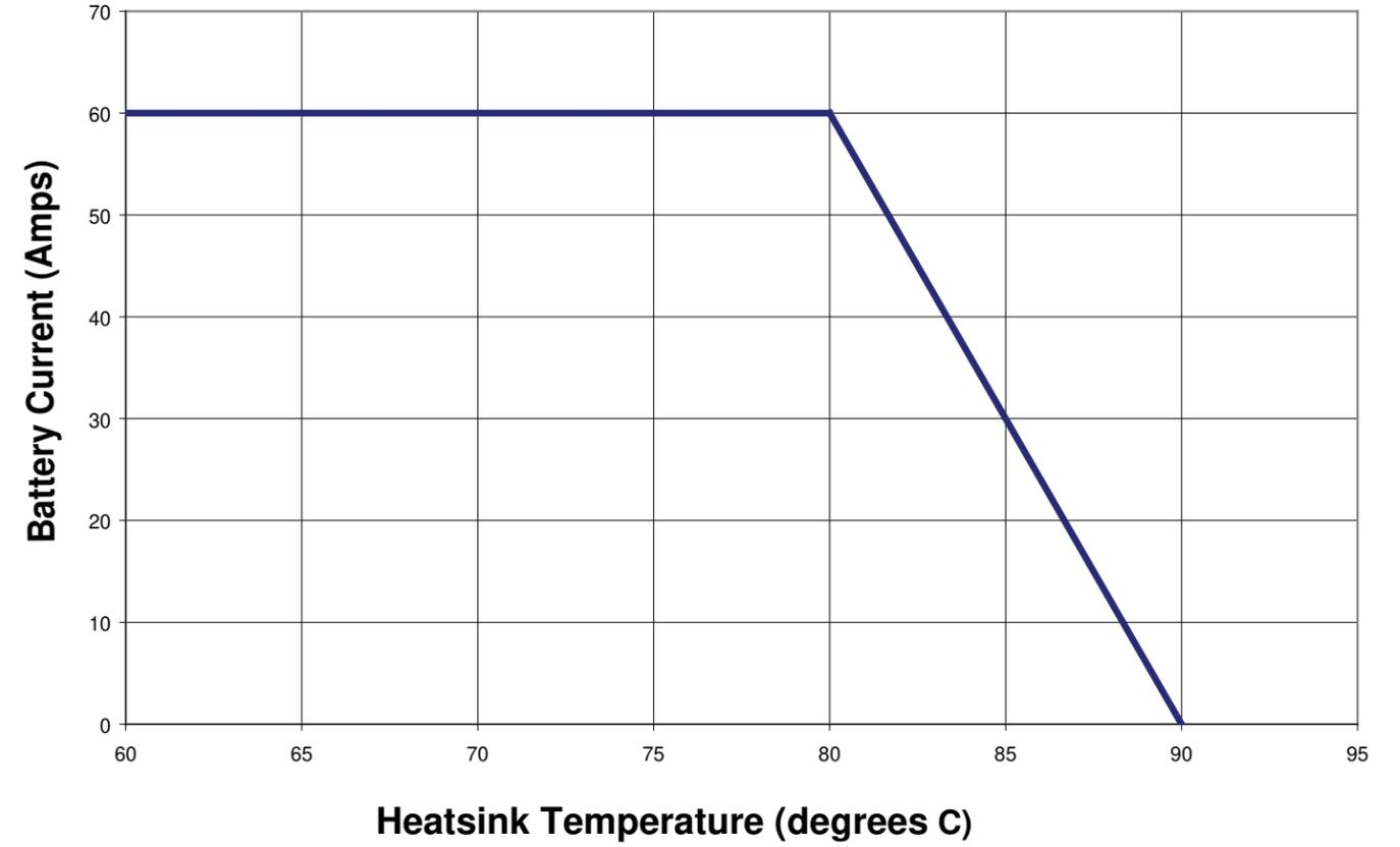
Figure 10-2. Battery Current vs. Heatsink Temperature
