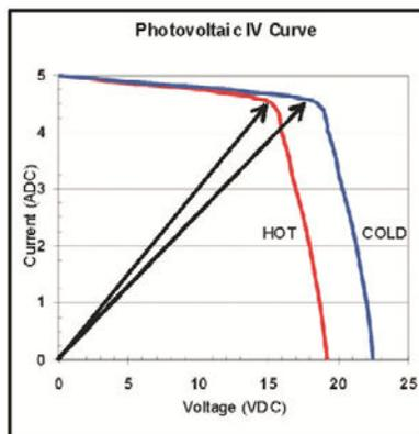
Additionally take note of the module performance IV curves for a 12V nominal PV module. It shows that under the hottest conditions the voltage is still high enough to provide charging current for the batteries.
