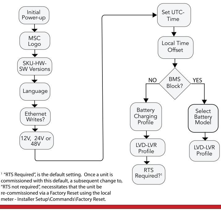
"RTS not required", necessitates that the unit be meter - Installer Setup\Commands\Factory Reset.
