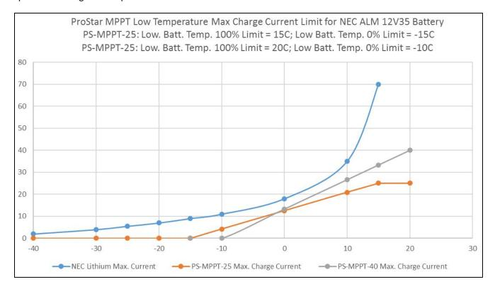
ProStar MPPT model PS-MPPT-25M Low Temp. Foldback Custom Settings. Low Battery Foldback High Limit = 15°C Low Battery Foldback Low Limit = -15°C
