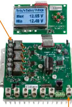
Large diameter, high torque, corrosion-resistant terminals
