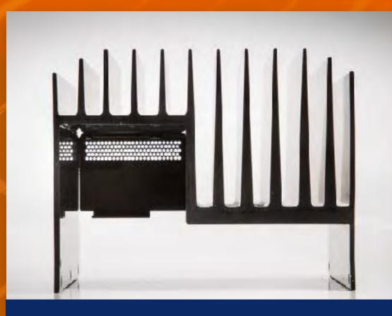
(LEFT) Morningstar's unique heat-sink assembly used in the TriStar controllers. Ordinary heat-sinks use flat metal fins. The extruded aluminum Morningstar heat-sink uses tapered fins, which greatly improves ambient air natural heat convection and helps eliminate the need for cooling fans.
