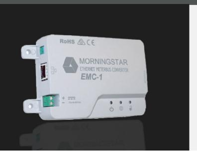
The Ethernet MeterBus Converter (model: EMC-1) provides the data and communications connection for Morningstar devices, between themselves, with surrounding systems, and with the outside environment through the internet. It's simple to connect to any compatible Morningstar product equipped with an RJ-11 Meterbus port (see the list of products at the table inside) to enable remote monitoring, custom programming, and access to future cloud-based data services.
