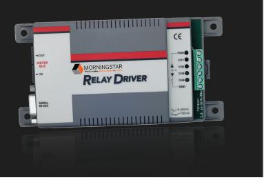
Morningstar's Relay Driver is a logic module which provides high level system control functions such as load control, generator start and alarm signaling. The product controls four independent relay driver outputs with battery voltage and other threshold settings in stand-alone mode or by reading digital data inputs from other Morningstar meterbus enabled devices in the system. The four channels can also be utilized as analog inputs to enable voltage threshold actions.
