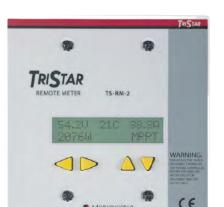
Remote Digital Display for the TriStar Family Controllers. The TS-RM-2 provides the same data display as the TS-M-2, except that it ships with 30 meters of cable and a flat faceplate. These features enable convenient mounting away from the controller.
