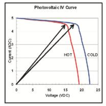
Additionally take note of the module performance IV curves for a 12V nominal PV module. It shows that under the hottest conditions the voltage is still high enough to provide charging current for the batteries.
