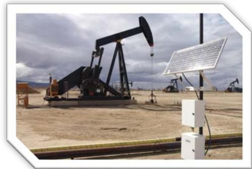
Our [SunSaver](#) and [SunKeeper](#) controllers are uniquely qualified for use in Oil & Gas Installations—the operating temperature of their internal circuitry is much lower than the auto-ignition temperature of most flammable gases and vapors. They are also well sealed and operate at low temperatures without the use of relays, thus preventing the high temperature arcing and sparking. Each product version has been certified and reaffirmed by an independent laboratory.
